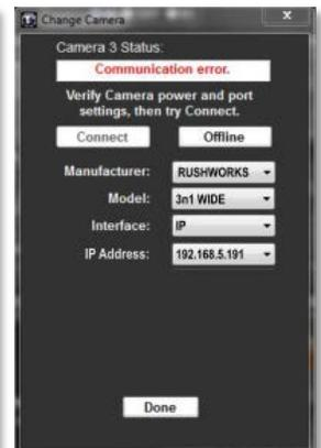
If you select the IP interface, many of the irrelevant entry fields will disappear and you'll then see only the entry fields for the camera's IP addresses - one for the PTZ camera (**Model: 3n1 PTZ**) and the other for the Wide Angle camera (**Model: 3n1 WIDE**).
