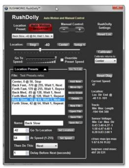
The control interface is similar to the Dynamic Auto Zoom setup for PTZ cameras, giving the operator precise control of start/stop positions, speed of travel, and multiple preset scripting.
