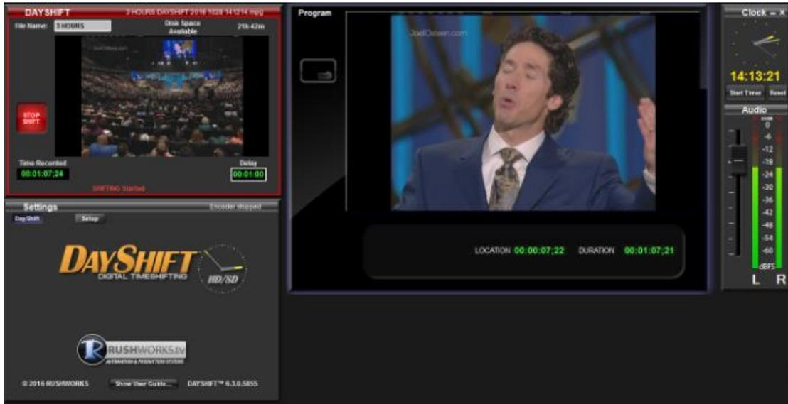
The **DAYSHIFT** user interface has different panels for controlling different functions. You can arrange these panels on the desktop however you wish.
