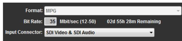
2) Select the **Bit Rate** for the encoding.
