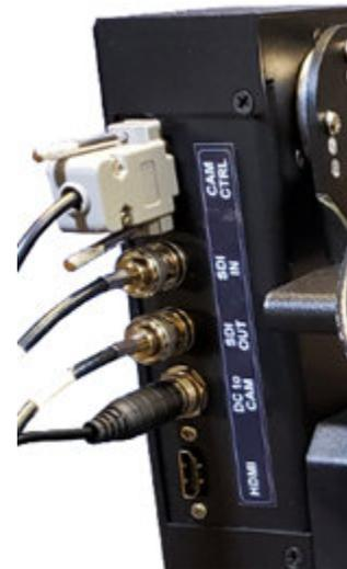
The SDI Out from the camera is then available on the BNC connector on the PTX chassis. If the camera provides an HDMI output, it's available on this chassis mount.
