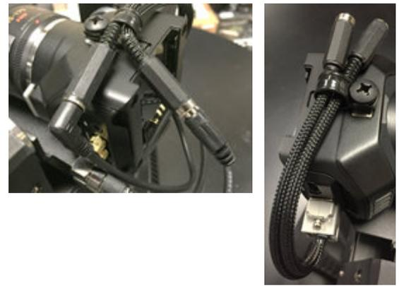
Then connect the LANC TO CAM and 12VDC TO CAM cables to the two cables/connectors from the HD15.
