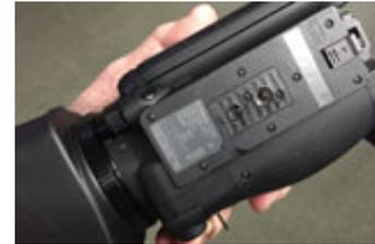
Some cameras, like the AJA RovoCam and Marshall CV models, have threaded mounts on both the bottom and the top ... so you can mount them “upside down” on the tilt plate then mount the PTX in an inverted position on truss or other structure if desired.
