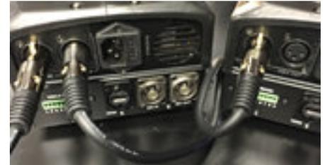
**VISCA Control:** Daisy-chain up to SEVEN PTX heads by connecting the RS422 OUT from the first to the RS422 IN of additional fixtures. **THE DMX ID MUST BE SET TO CHANNEL 1 ON ALL SEVEN FIXTURES!** The DMX/VISCA ID (DIP switch) must be set to 1 - 7 on the respective fixtures.
