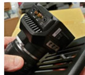
Tighten the thumbscrew to secure the camera, but only tight enough that the camera can slide forward and backward along the slot.
