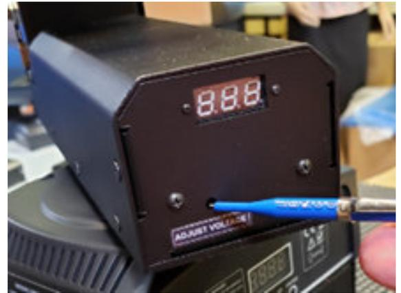
Use the built-in voltage display meter to confirm your settings during output adjustment.
