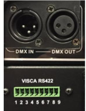
The Camera is a camera or camcorder connected to the tilt plate on the PTX fixture. Cameras are controlled using the internal protocols supported by the PTX. These include LANC, Panasonic Remote and VISCA connections.
