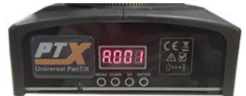
To change the DMX ID, click the ENTER button beneath the LED display and you'll see red dots separating the ID segments.
